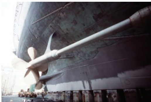
Courtesy of the National Archives and Records Administration Propeller shaft of the battleship USS Missouri
