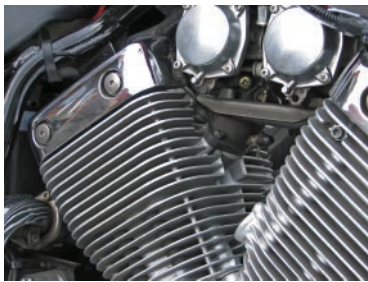
© GDragan/iStock/Thinkstock Cooling fins on a motorcycle engine
